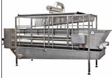
Figure 12 - Continuous industrial fish thawing equipment (Carnitech)
