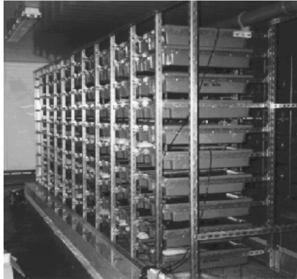
Vertical stack system using Seafish containers
