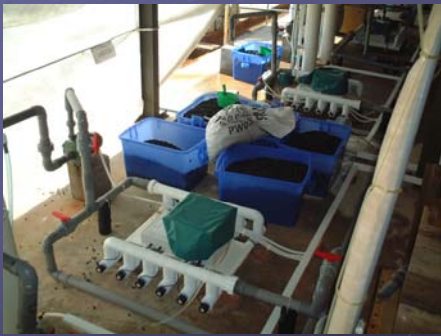
Boxes of charcoal for filters and UV light tubes for sterilising water
