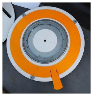
Rather than attach the printed paper circle to the base of my scope I decided to fit a plastic circle between the Lazy Susan bearing and the outside of the base. The setting circle "ring" is held in place by three plastic buttons. These are the same plastic buttons that the base would have originally rotated on, and which were left in place when the previous owner added the Lazy Susan bearing.
