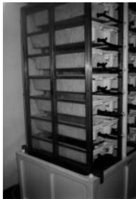
Containers supported on stainless steel frame
