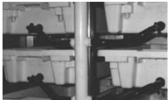
Flexible drain tubes and central drain
